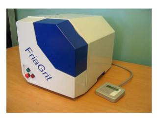
A method measuring the impact strength of diamond grits, based on the principle that the friability test will be applied until 50% of the grits are broken. The time needed to reach this stage will be considered.
