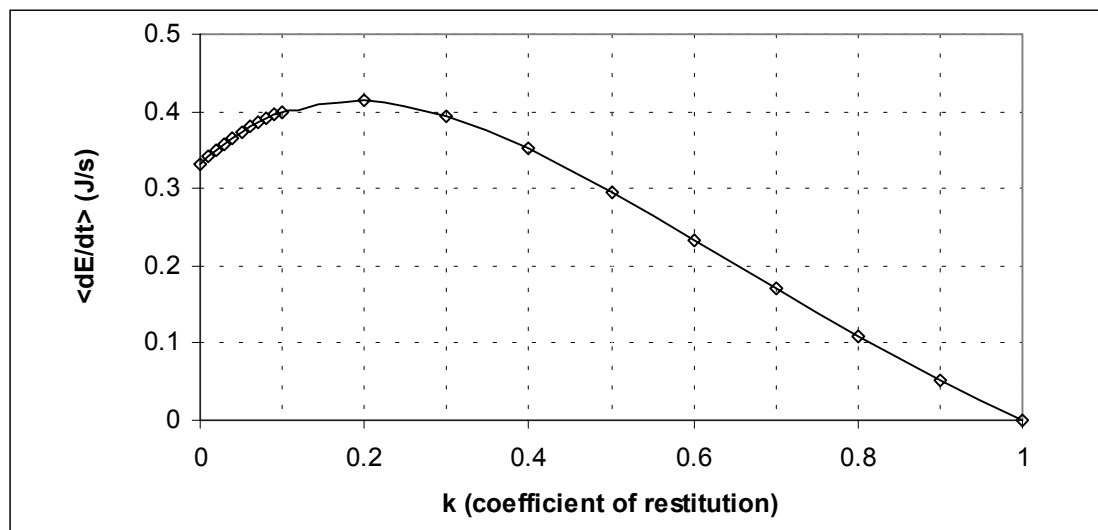
Fig. 2: effect of k on energy transfer rate (all other parameters equal to the default values of §2)
